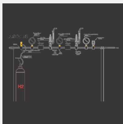
Pressure Reducing System
